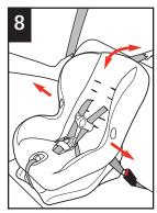
With weakest hand at belt path, tilt and push the child restraint forward and back, and from side to side. If the seat belts do not loosen, your child restraint should be secure.
